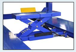
Electro / Hydraulic Jacking Bridges Electric / Hydraulic jacking bridges with their own control box are also fitted. These allow for the vehicle to be lifted off the platform.
