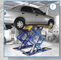
For optional inground installation, spacer boxes are supplied to allow the lift to be lowered with the platforms extended.
