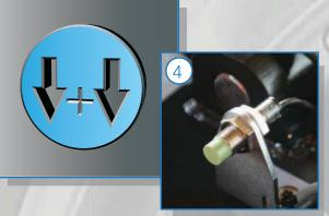
Two Stage lowering for the safety(optior It is equipped with an anticrushing safety device that lockhe lift during descent at 150mm above the ground; lowering will not continue until a further command is given from the control panel. A beeper will then sound throughout the final lowering phase.
